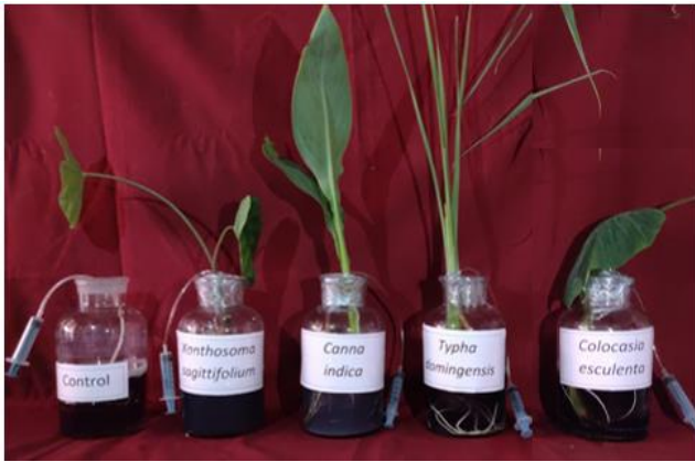
Fig. 2 Experimental setup for estimating the radial oxygen loss (ROL)
