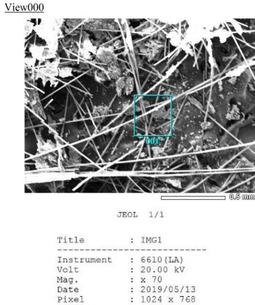
Fig. 10 Analysis of sealant powder recovered from the surface of outlet disc membranes by SEM
