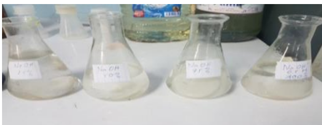
Fig. 5 Treatment of membranes with NaOH
