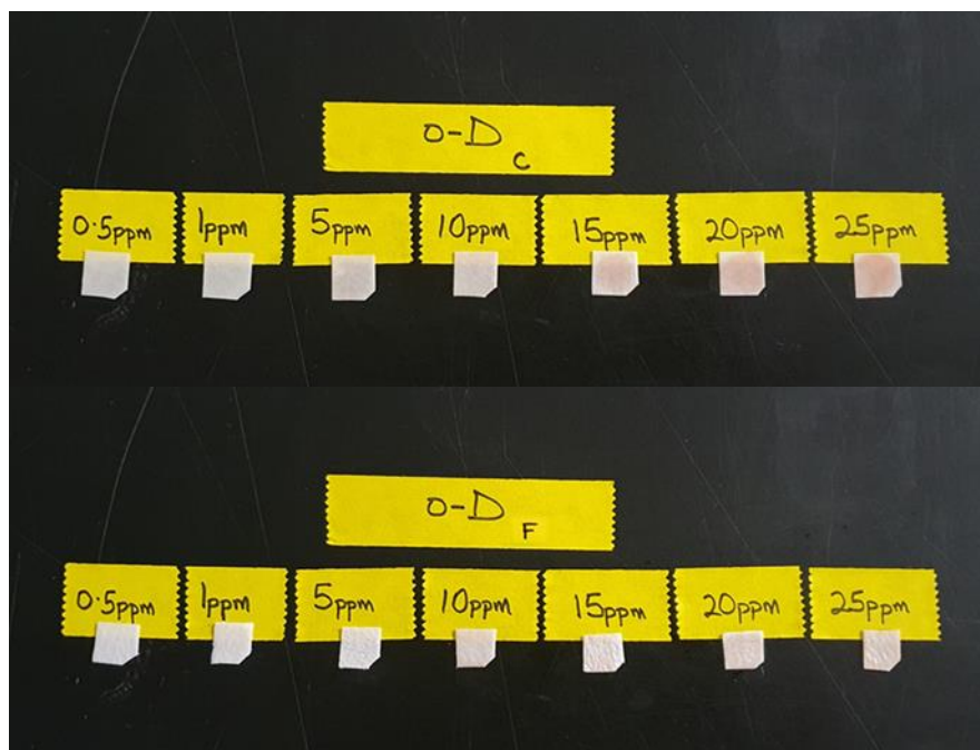
Fig. S5. o -D paper-based test strips coloration after 2 months of storage
