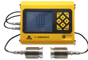
Fig. 8 The crack instrument
