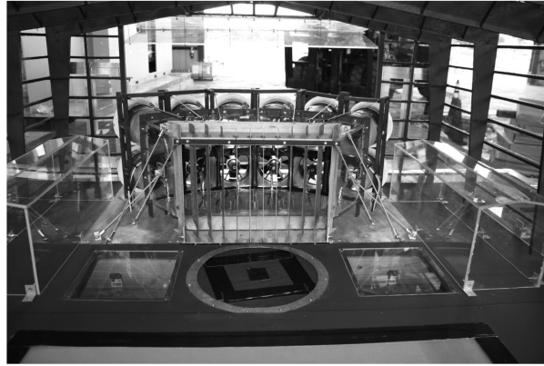
Fig. 1 Small-scale 12-fan Wall-of-Wind (WoW)
