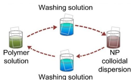
Scheme 2 Illustration of the LbL assembly of IONP/polyelectrolyte nanocomposite
