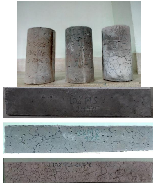
Fig. 6 Cracks in concrete specimens after heating
