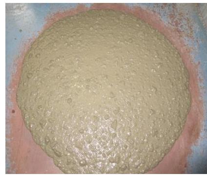
(b) Slump flow
