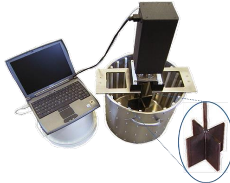
Fig. 5 ICAR Rheometer set up and testing
