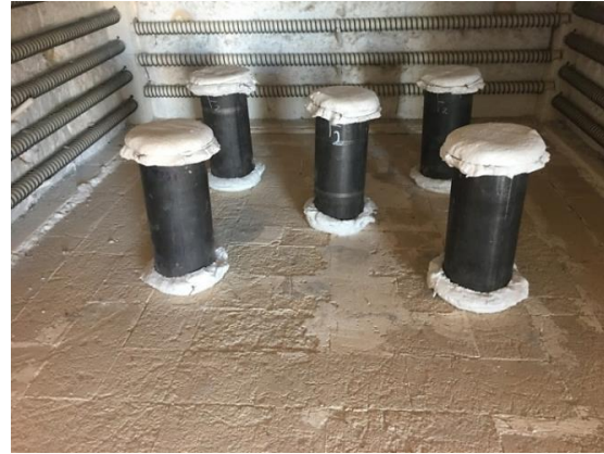
Fig. 5 Setup of column specimens inside the furnace before exposure to fire
