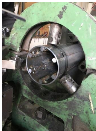
Fig. 3 Machining of steel tubes
