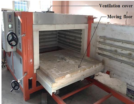
Fig. 4 The utilized furnace
