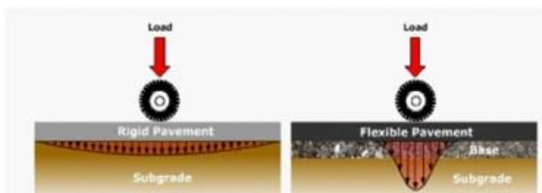
Fig. 2 Deflection of rigid and flexible pavement
