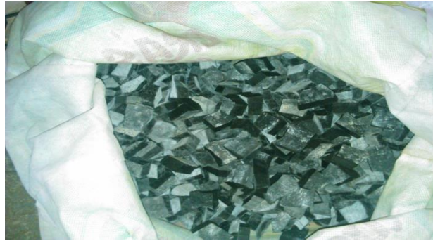
Fig. 1 Reclaimed rubber used for concrete
