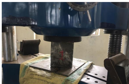
Fig. 4 Compressive strength test on cubes using universal testing machine
