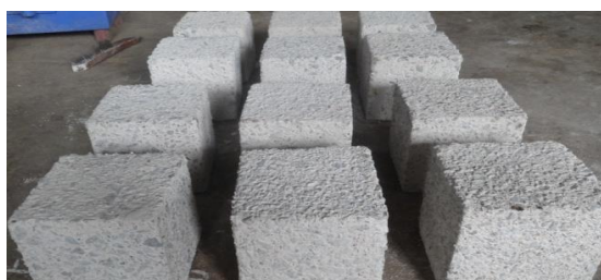
Fig. 3 Concrete cubes after acid attack
