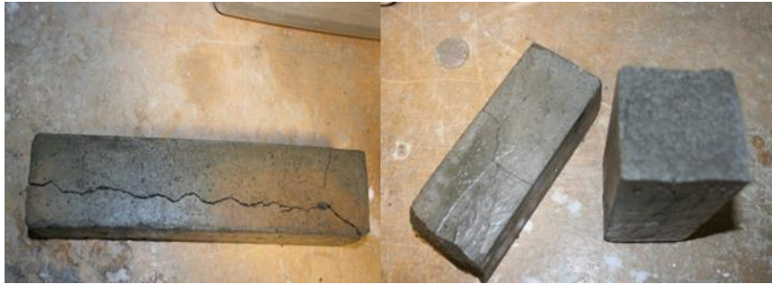
Fig. 7 The specimens after significant number of freezing and thawing cycles
