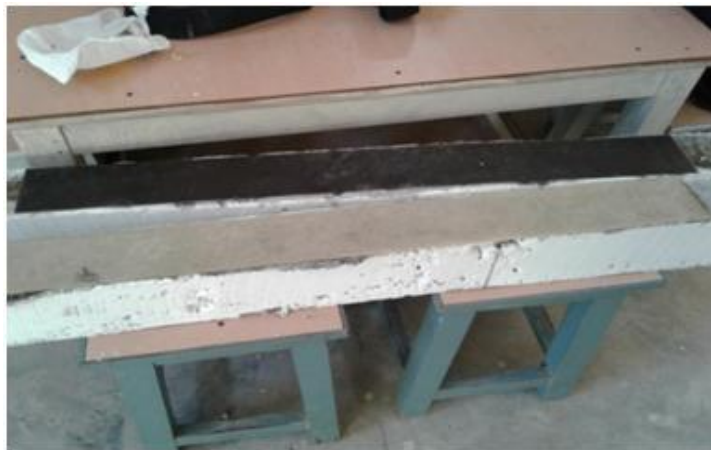
Fig. 2 FRP laminates on the tension side of the beam
