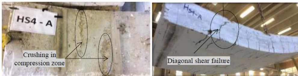
Fig. 16 Mode of failure in slab HS4-A
