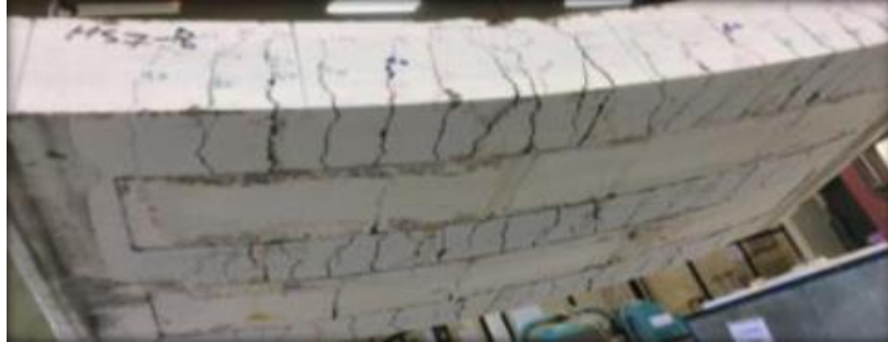
Fig. 24 Mode of failure in slab HS7-B
