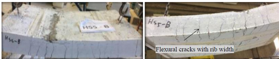
Fig. 23 Mode of failure in slab HS5-B
