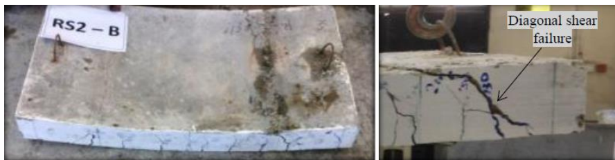
Fig. 21 Mode of failure in slab RS2-B
