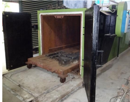
Fig. 3 Specimen in steam curing chamber
