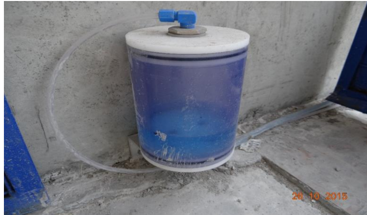
Fig. 4 Hydraulic cell level water pressure reservoir
