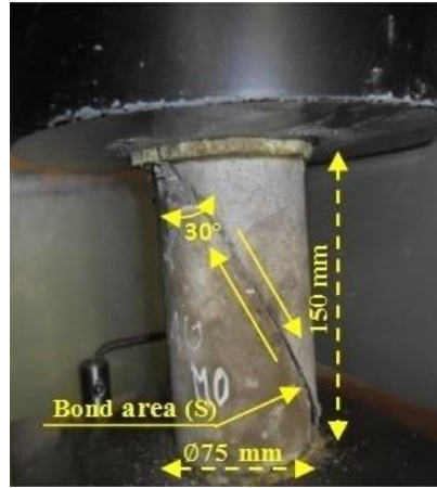
Fig. 3 slant-shear specimen under compression testing
