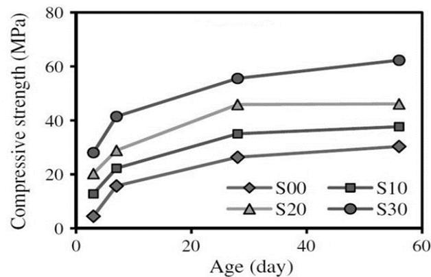
Fig. 6 Effect of different percentage of GGBS on compressive strength development of the geopolymer concrete (Pradip and Prabir 2014)
