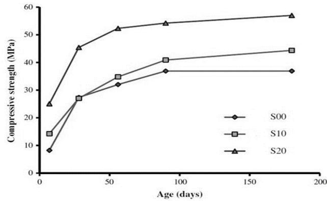
Fig. 5 Compressive strength variation of geopolymer concrete with different slag (Deb *et al.* 2014)
