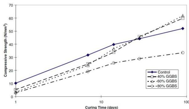
Fig. 4 Effect of GGBS on compressive strength development (Khatib and Hibbert 2005)
