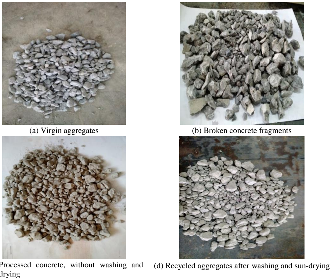
Fig. 3 Aggregates before and after processing
