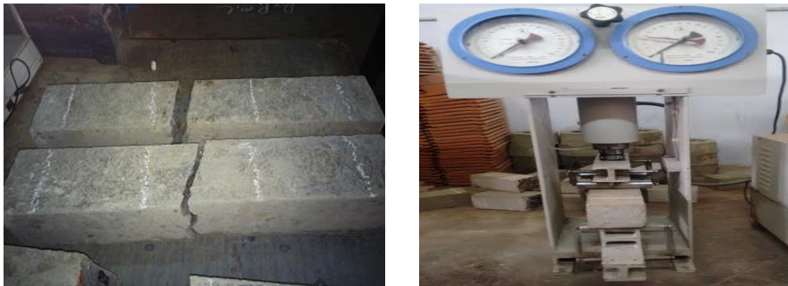
Fig. 13 Flexural Strength arrangement and cracked beams
