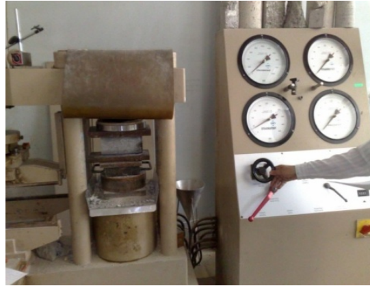
Fig. 3 Brazilian test for tensile strength measurements
