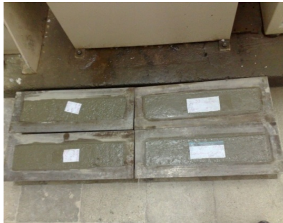
Fig. 1 Prismatic specimens for determination of flexural and compressive strengths
