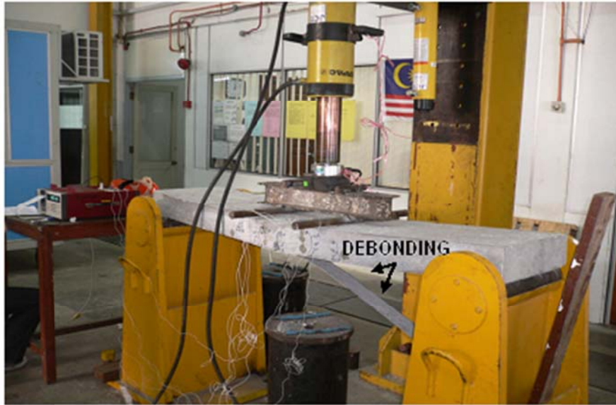
Fig. 4 CFRP debonding at the CFRP/concrete interface under line load
