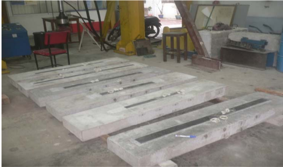
Fig. 1 RC one-way slab strengthened by different lengths and width of CFRP
