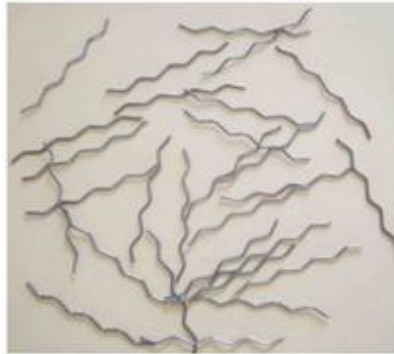
Fig. 1 Crimped steel fibres
