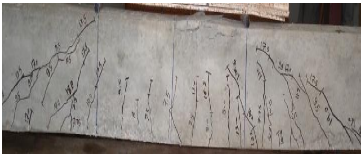
Fig. 4 Flexural – shear failure of the solid beam
