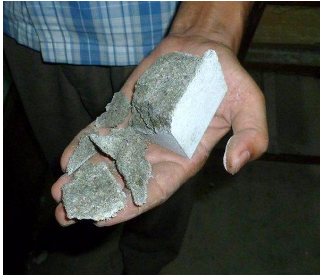
Fig. 6 Final failure pattern of modified mortar cube specimen
