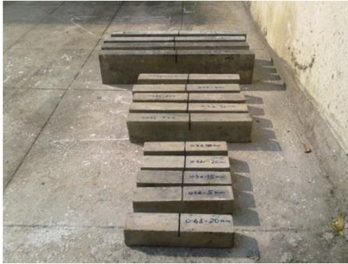
Fig. 4 Typical notched beam specimens
