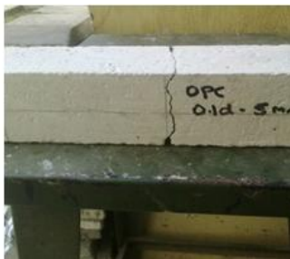
(a) NSC - 250 × 50 × 50 (notch depth = 5 mm)
