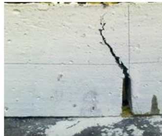
(b) HSC - 500 × 50 × 100 (notch depth = 20 mm)
