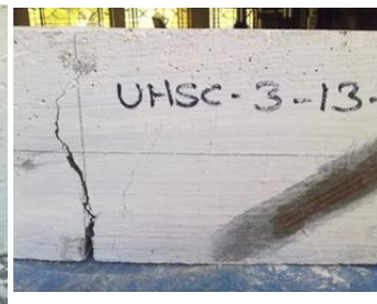
(c) UHSC - 650 × 50 × 130 (notch depth = 13 mm)
