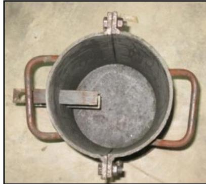
Fig. 4 Steel mould with flat plates
