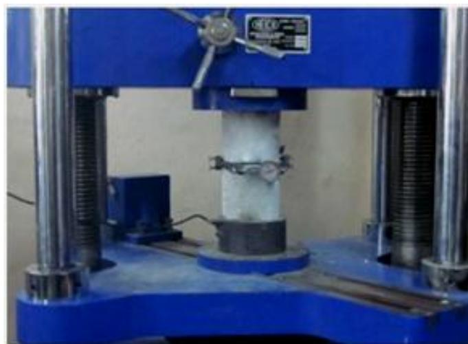
Fig. 12 Test set-up for Poisson's ratio
