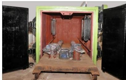
Fig. 3 Specimens in steam curing chamber
