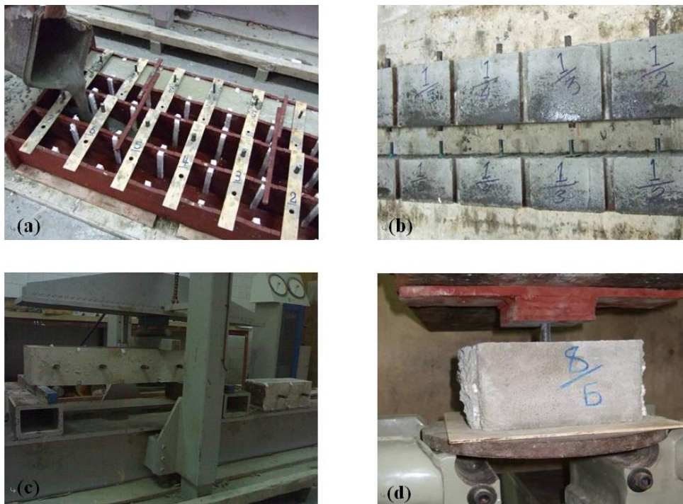
Fig. 5 Preparation and testing of push-out test specimens
