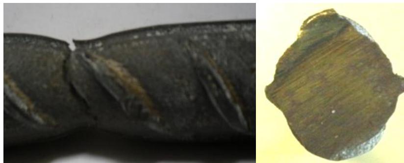
Fig. 10 Failure point of the non-corroded bar B2T-1-2 with necking phenomena
