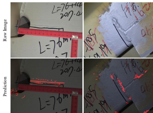
Fig. 7 Raw images and prediction results obtained from dataset D1
