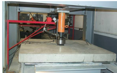
Fig. 5 Experimental slab model under loading (Agbossou et al. 2008)
