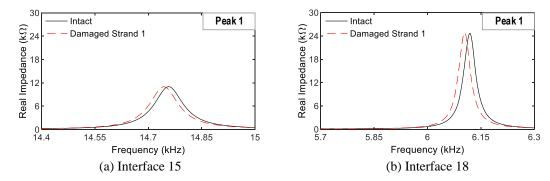
Fig. 22 Impedance signatures of Interfaces 15-18 zoomed in Peak 1's frequency range: Strand 1 breakage
