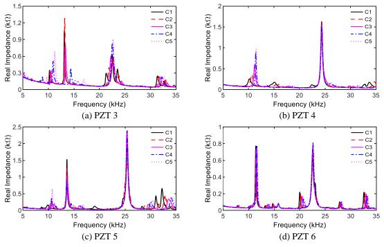
Fig. 31 Impedance responses of four PZT-patch sizes under compression
