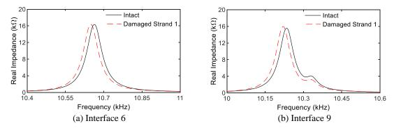
Fig. 16 Impedance signatures of Interfaces 6-9 zoomed in Peak 1's frequency range: Strand 1 breakage
