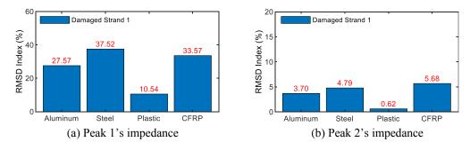
Fig. 5 Sensitivities of impedance signatures of four interface materials for damage detection
