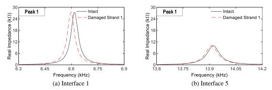
Fig. 13 Impedance signatures of Interfaces 1-5 zoomed in Peak 1's frequency range: Strand 1 breakage
