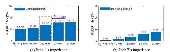
Fig. 20 Sensitivities of impedance signatures of Interfaces 10-14 for damage detection
