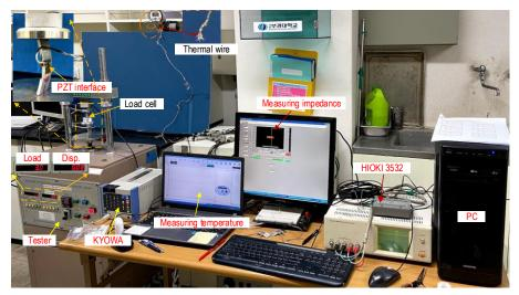
Fig. 24 Test set-up of PZT interface in compression tester for impedance measurement
