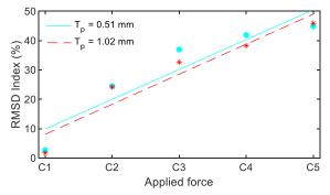
Fig. 30 Sensitivity of experimental impedance responses versus different thicknesses of PZT sensors under compression
