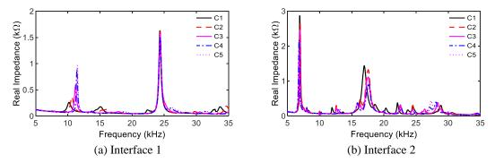
Fig. 33 Experimental impedance responses measured from different thicknesses of hoop interfaces under compression
