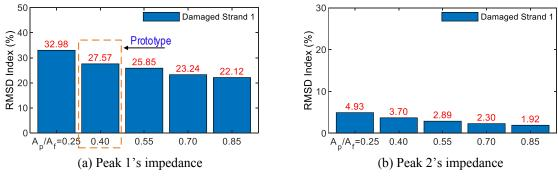
Fig. 11 Sensitivities of impedance signatures of PZTs 5-9 for damage detection
