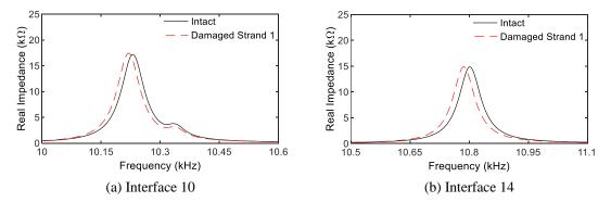
Fig. 19 Impedance signatures of Interfaces 10-14 zoom in Peak 1's frequency range: Strand 1 breakage
