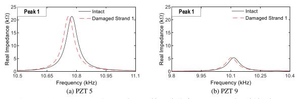
Fig. 10 Impedance signatures of PZTs 5-9 zoomed in Peak 1's frequency range: Strand 1 breakage
