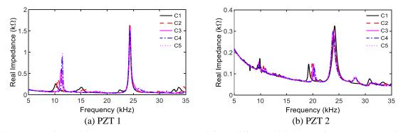
Fig. 29 Experimental impedance responses measured from different thicknesses of PZT sensors under compression
