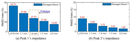
Fig. 14 Sensitivities of impedance signatures of Interfaces 1-5 for damage detection
