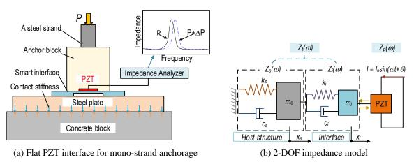
Fig. 1 Concept of impedance measurement via PZT interface at prestressed anchorage
