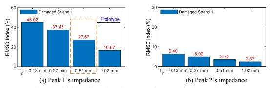
Fig. 8 Sensitivities of impedance signatures of PZTs 1-4 for damage detection
