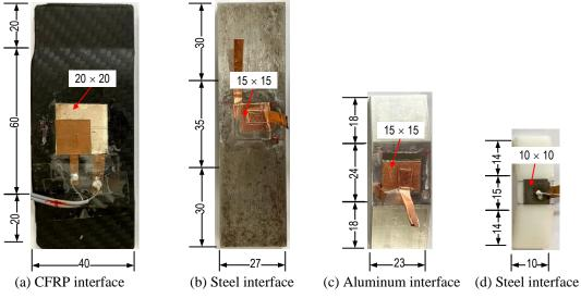
Fig. 25 Four different material types of PZT interfaces
