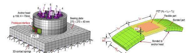
Material and geometric properties of hoop-type PZT interface for damage-sensitive impedance... 133
