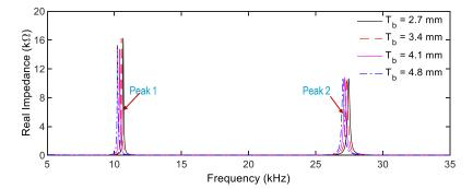
Fig. 15 Impedance signatures of Interfaces 6-9 in the range 5-35 kHz: intact state
