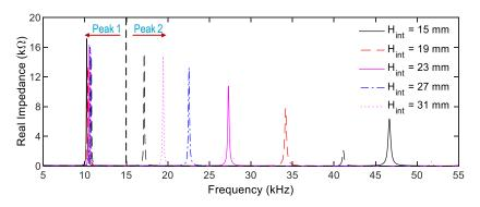
Fig. 18 Impedance signatures of Interfaces 10-14 in the range 5-55 kHz: intact state
