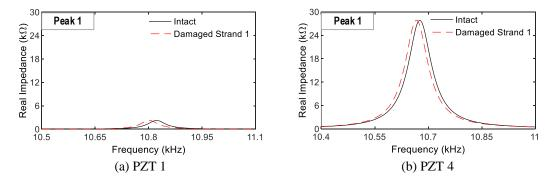
Fig. 7 Impedance responses of PZTs 1-4 zoomed in Peak 1's frequency range: Strand 1 breakage
