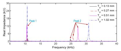
Fig. 6 Impedance signatures of PZTs 1-4 in the range 5-40 kHz: intact state
