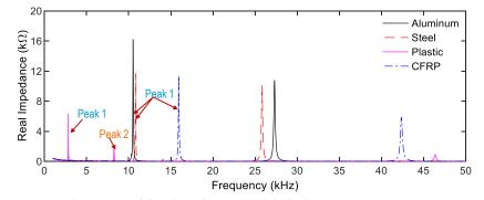
Fig. 3 Impedance signatures of four interface materials in frequency range 1-40 kHz: intact state
