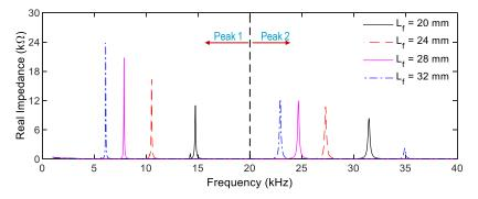
Fig. 21 Impedance signatures of Interfaces 15-18 in the range 2-40 kHz: intact state
