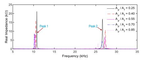
Fig. 9 Impedance signatures of PZTs 5-9 in the range 5-35 kHz: intact state
