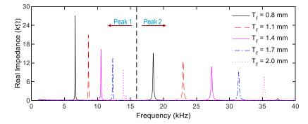
Fig. 12 Impedance signatures of Interfaces 1-5 in the range 2-40 kHz: intact state
