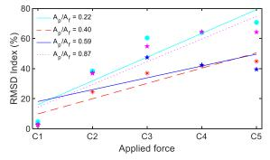
Fig. 32 Sensitivities of impedance responses of four PZT-patch sizes for stress monitoring
