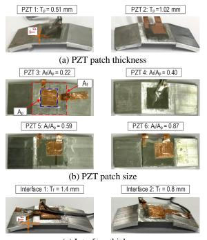
(c) Interface thickness Fig. 26 Interface thickness, PZT-patch thickness, and PZT-patch covering area
