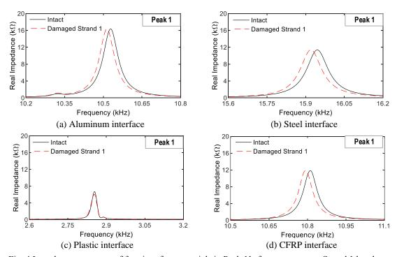
Fig. 4 Impedance responses of four interface materials in Peak 1's frequency range: Strand 1 breakage
