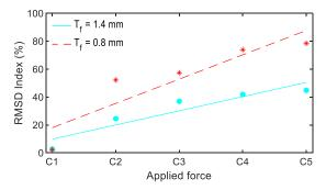
Fig. 34 Sensitivity of experimental impedance responses versus different thickness of hoop-interface under compression
