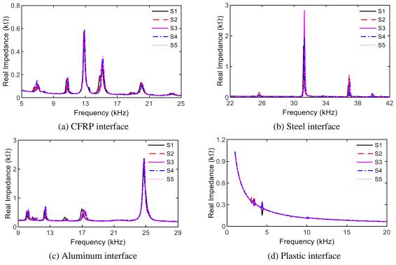
Fig. 27 Impedance responses of four interface materials under compression
