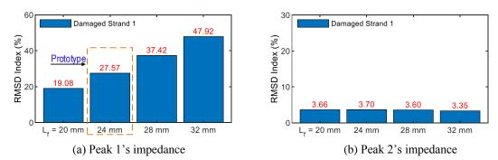
Fig. 23 Sensitivities of impedance signatures of Interfaces 15-18 for damage detection
