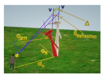
Fig. 7 Example of deflection angle in a wind tower
