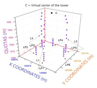
Fig. 9 result of the quotas and coordinates (x,y) of the transverse welds from the reference points
