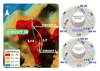
Fig. 5 Scheme of the circuits carried out with the geometric leveling
