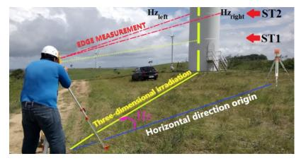
Fig. 6 Procedures for measuring transverse welds
