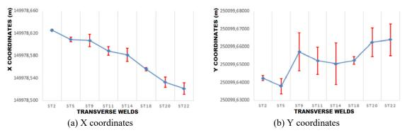
Fig. 10 Combined model: x and y coordinates of the transverse welds
