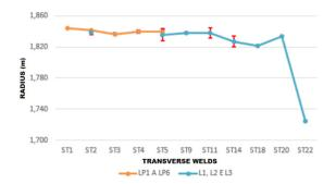
Fig. 11 Radii of circular sections from hexagon and triangle reference points
