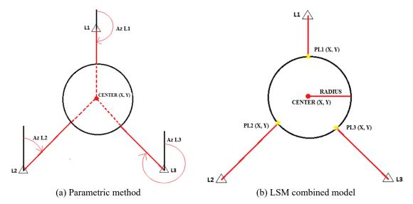
Fig. 8 Example of determining the coordinates of the center (x, y) of the circular section of the transversal weld
