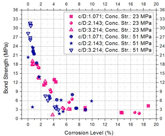
(a) Data from Yalciner *et al.* (2012) (Pull-out test) – used for model development and testing
