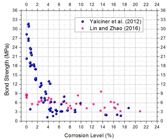
(b) Data from Yalciner *et al.* (2012) (Pull-out test) and Lin and Zhao (2016) (Flexural test)
