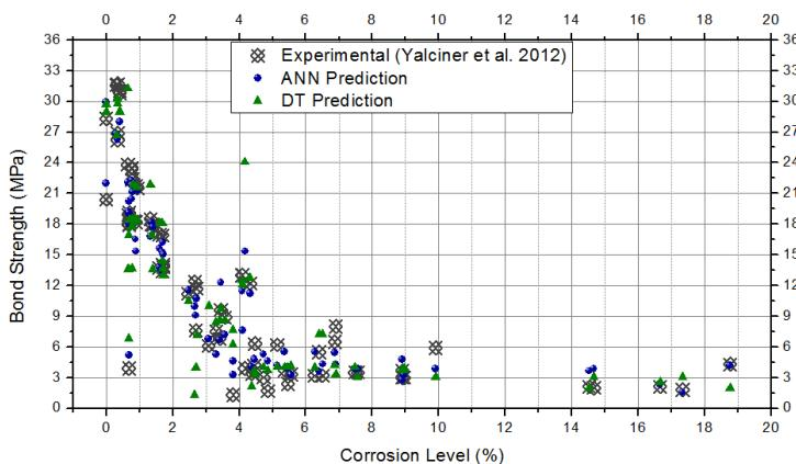
Fig. 5 Variable plot of experimental bond strength (Yalciner *et al.* 2012) and model (ANN, DT) predictions
