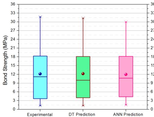
Fig. 6 Box-and-whisker plot of experimental bond strength (Yalciner *et al.* 2012) and model (ANN, DT) predictions
