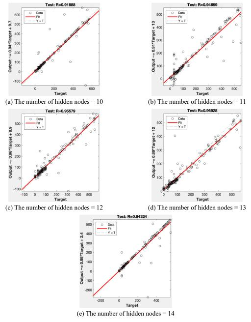
Fig. 5 The degree of fit of the first NN model (the number of hidden nodes = 10, 11, 12, 13, 14)
