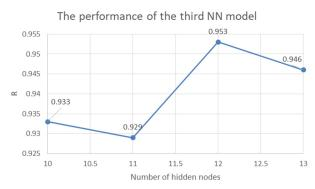
Fig. 12 The tests correlation coefficients of the different hidden layers of the third NN model
