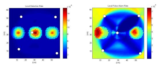
Fig. 11 Local detection (left) and false alarm rate (right) with five-sensor optimal arrangement for a fixed global detection rate of  $P_D = 0.95$  and correlation level  $b_1 = 0.7$
