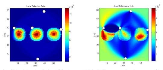
Fig. 10 Local detection (left) and false alarm rate (right) with five-sensor optimal arrangement for a fixed global detection rate of  $P_D = 0.95$  and correlation level  $b_1 = 0.4$
