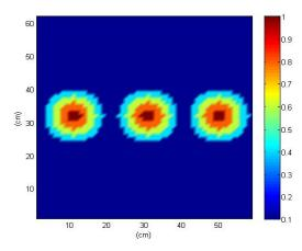
Fig. 8 Non-uniform damage distributions over the plate with three riveted holes
