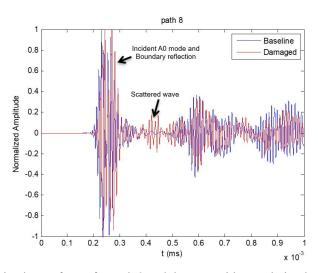
Fig. 19 Received waveforms for path 8 and the case with correlation level  $b_1 = 0.2$
