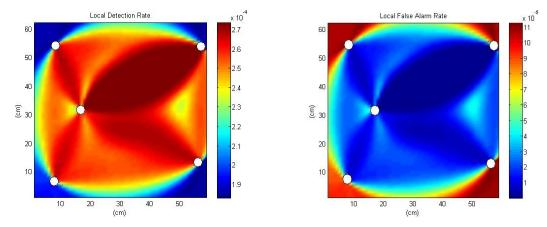
Fig. 6 Local detection (left) and false alarm rate (right) with five-sensor optimal arrangement for a fixed global detection rate of  $P_D = 0.95$  and correlation level  $b_1 = 0.7$
