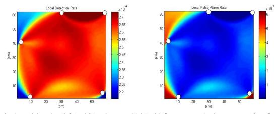
Fig. 4 Local detection (left) and false alarm rate (right) with five-sensor optimal arrangement for a fixed global detection rate of  $P_D = 0.95$  and correlation level  $b_1 = 0.2$
