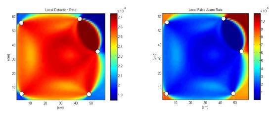
Fig. 5 Local detection (left) and false alarm rate (right) with five-sensor optimal arrangement for a fixed global detection rate of  $P_D = 0.95$  and correlation level  $b_1 = 0.4$
