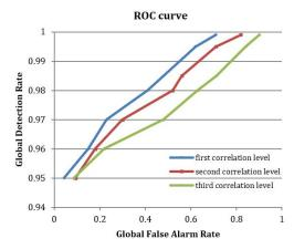
Fig. 13 ROC curve for different levels of correlation for non-uniform damage distributions
