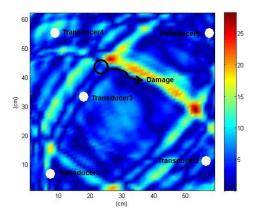
Fig. 23 Delay and sum imaging result with optimal arrangement for global detection rate of  $P_D = 0.95$  and correlation level  $b_1 = 0.7$
