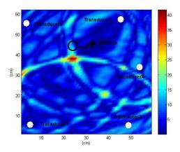
Fig. 22 Delay and sum imaging result with optimal arrangement for global detection rate of  $P_D = 0.95$  and correlation level  $b_1 = 0.4$
