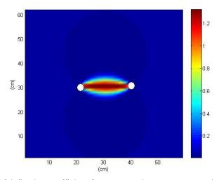
Fig. 3 Spatial map of deflection coefficient for two-transducer arrangement in pitch-catch scheme
