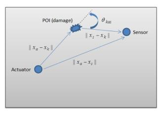
Fig. 1 Distances between actuator-POI-sensor
