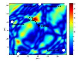
Fig. 21 Delay and sum imaging result with optimal arrangement for global detection rate of  $P_D = 0.95$  and correlation level  $b_1 = 0.2$
