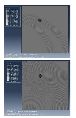
Fig. 18 Wave propagation in presence of a through-thickness hole
