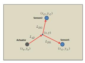
Fig. 20 Propagation paths from an actuator to damage to sensors
