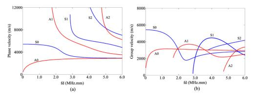
Fig. 15 Dispersion curve of lamb modes for aluminium plate (a) phase velocity; (b) group velocity (Liu *et al.* 2012)
