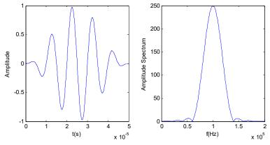
Fig. 14 A 5 cycle tone burst signal and its frequency response
