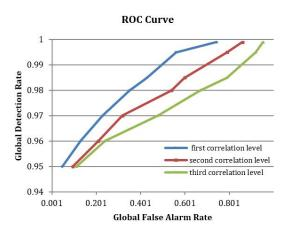
Fig. 12 ROC curve for different levels of correlation for uniform damage distributions
