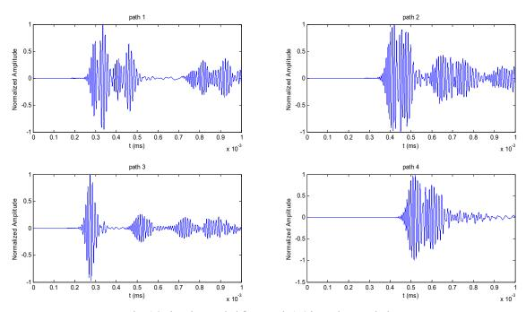
Fig. 16 Signal recorded from path 1-4 in undamaged plate
