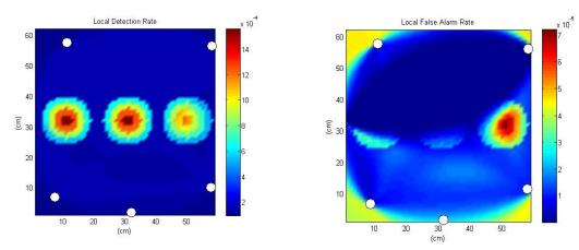
Fig. 9 Local detection (left) and false alarm rate (right) with five-sensor optimal arrangement for a fixed global detection rate of  $P_D = 0.95$  and correlation level  $b_1 = 0.2$
