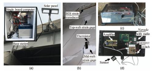
Fig. 3 Highlights of Telegraph Road Bridge instrumentation: (a) base station with solar panel used for power; (b) installation of strain sensors (BDI strain transducer on slab and metal foil gages on girders); (c) wireless sensor enclosure for strain gage data collection magnetically mounted to steel girder flange; and (d) internal components of wireless sensor node. (Figure from Hou *et al.* 2020a)
