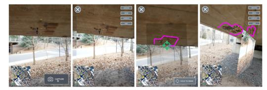
Fig. 4 Screen shots of the SHM management system developed for the Streicker Bridge. (a) Example of the initial capture scene; (b) as (a) but with the annotation screen; (c) example of annotation being taken on the point cloud, (d) the annotation projected back onto the image for offsite viewing. (From Napolitano *et al.* 2019)
