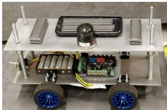
Fig. 2 Vehicle to induce vibration in the bridge
