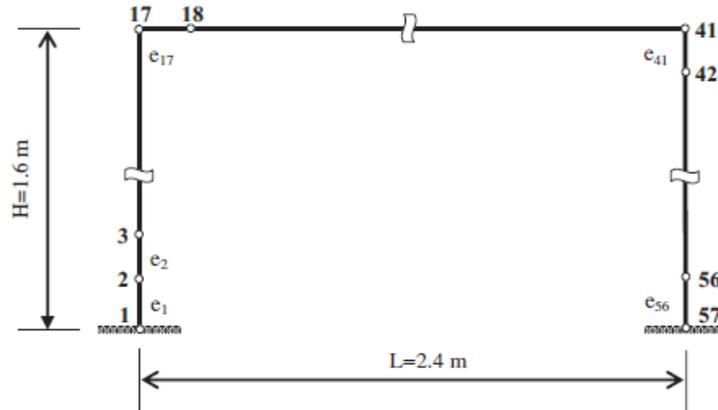
Fig. 6 A two-dimensional portal frame with 56 elements
