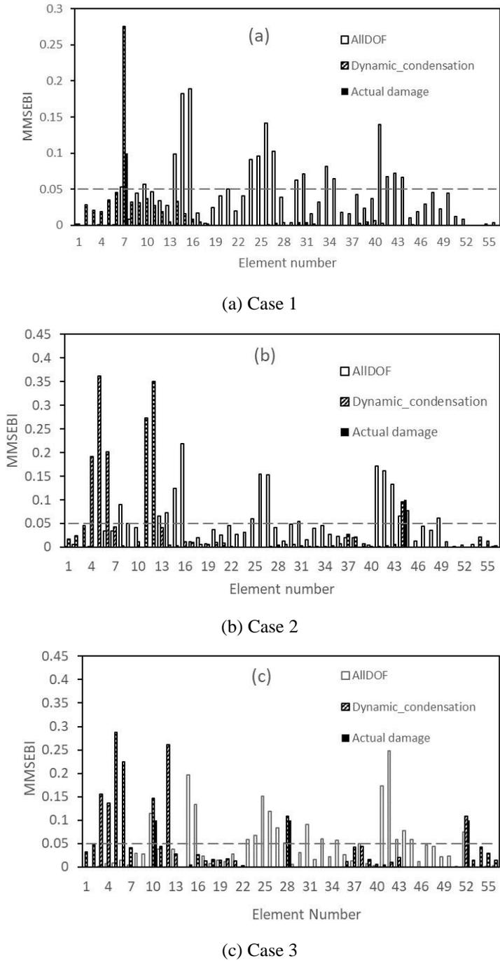
Fig. 8 Damage index values in the 56-element frame for 4 modes with considering 3% noise
