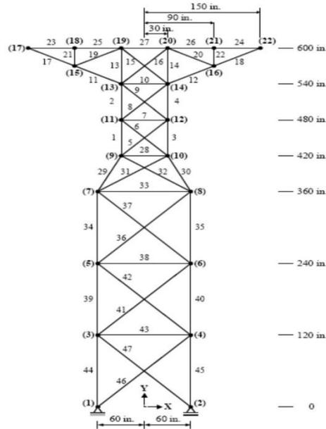
Fig. 1 A forty-seven-bar planar power line tower
