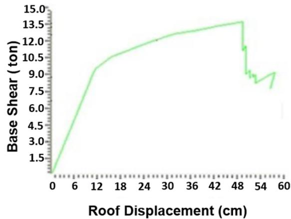
Fig. 1 Pushover diagram of a frame
