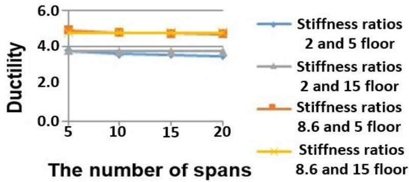
Fig. 3 Comparing the ductility by changing the number of spans
