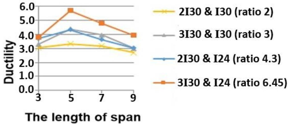
Fig. 5 Comparing the ductility by changing the length of span
