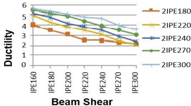
Fig. 2 Comparing the ductility by changing the column to beam moment of inertia
