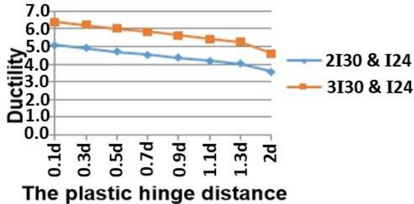
Fig. 7 Comparing the ductility by changing the plastic hinge distance from the column
