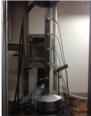
Fig. 4 Experimental specimen and sensor locations
