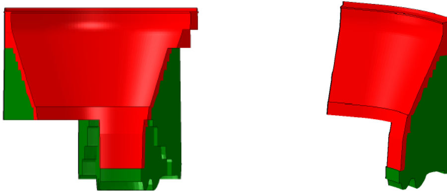
Fig. 14 Elastic modulus distribution in the arch-gravity dam (original value in green; reduced value in red)
