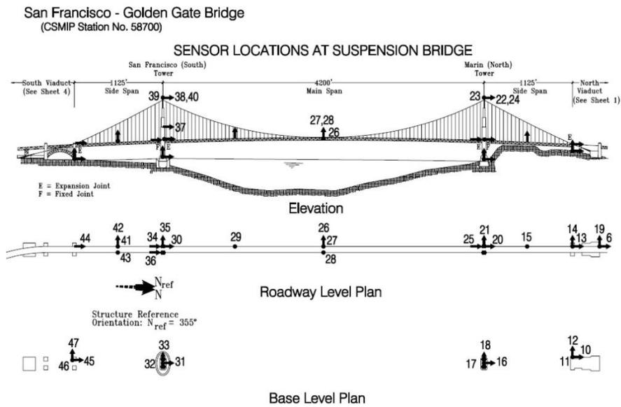
Fig. 5 Golden Gate bridge instrumentation (<http://www.strongmotioncenter.org>)
