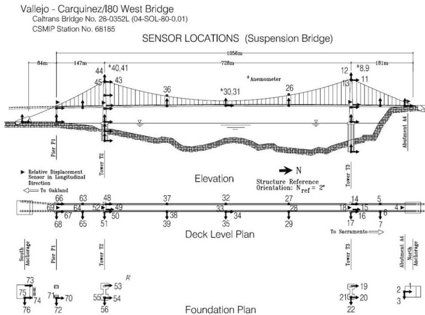
Fig. 8 Alfred Zampa bridge instrumentation (<http://www.strongmotioncenter.org>)
