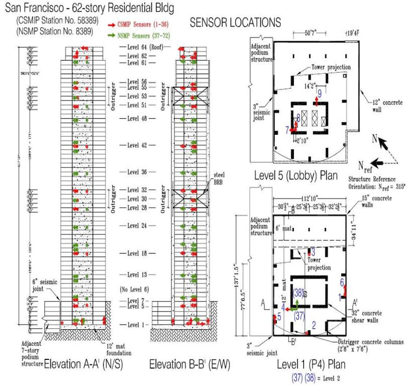
Fig. 4 One Rincon Hill Tower instrumentation (<http://www.strongmotioncenter.org>)
