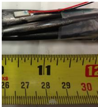
Fig. 5 Installed PZT transducers (Farhidzadeh 2014)
