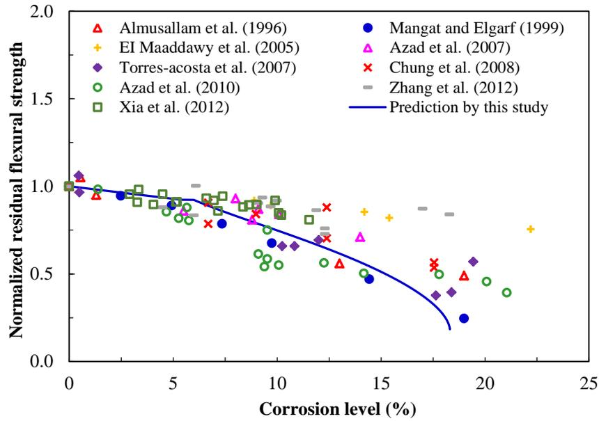
Fig. 1 Flexural strength deterioration versus corrosion level compared with published experimental data available
