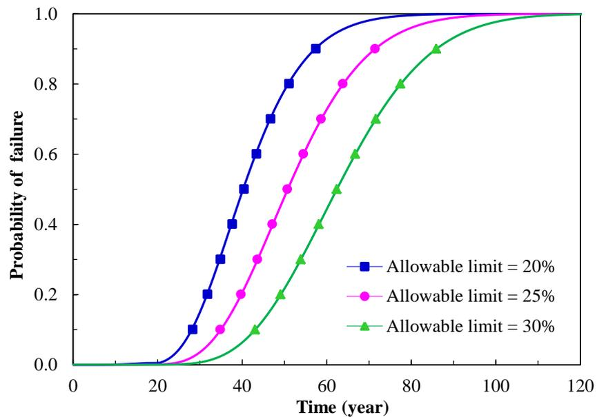
Fig. 2 Probability of structural failure over time for various allowable flexural strength deterioration limits
