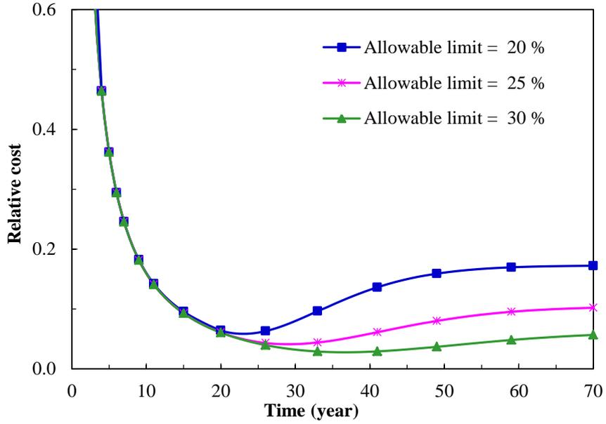
Fig. 3 Expected relative costs over repair time interval with discounting of an annual rate of 5% as a function of repair time for various allowable flexural strength deterioration limits
