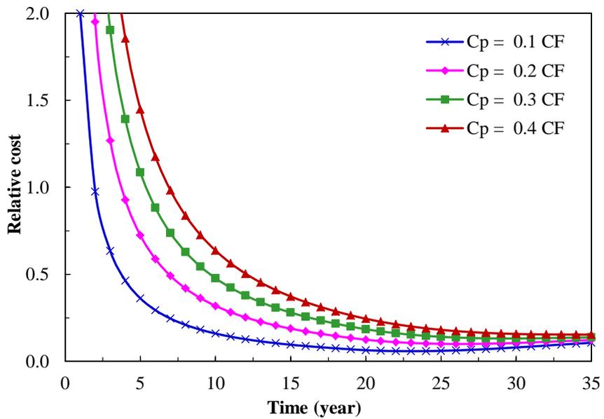
Fig. 4 Expected relative costs as a function of repair time for various preventive maintenance costs  $C_p$  in relation to corrective maintenance cost  $C_F$
