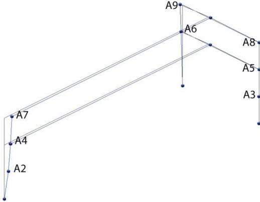
Fig. 3 Mode shape 1 –  $f_1=4.72$  Hz
