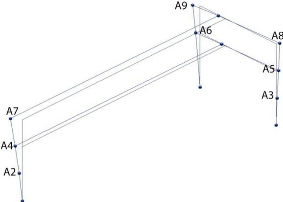
Fig. 5 Mode shape 3 –  $f_3=7.05$  Hz
