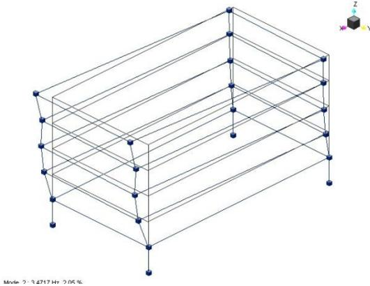
Fig. 10 Mode shapes 2 –  $f_2=3.48$  Hz
