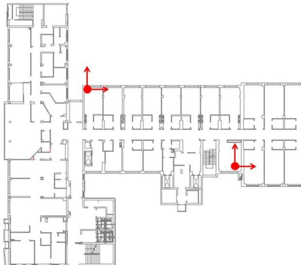
Fig. 8 Typical Sensor layout - 1st floor
