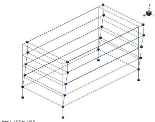
Fig. 9 Mode shapes 1 –  $f_1=2.88$  Hz
