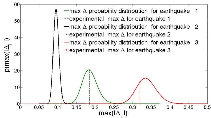
Fig. 6 Probability density functions and experimental values of maximum drifts
