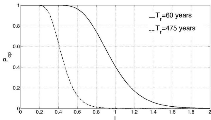
Fig. 13 Operational curves for seismic input from Italian Technical Code at 50 years and 475 years
