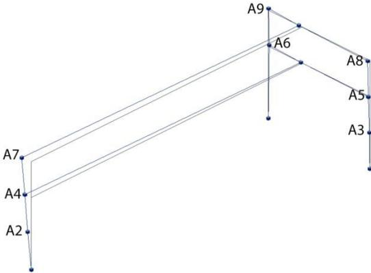
Fig. 4 Mode shape 2 –  $f_2=5.35$  Hz
