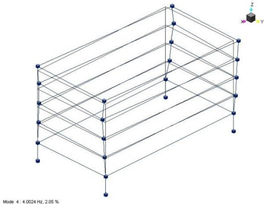
Fig. 11 Mode shapes 3 –  $f_3=4.00$  Hz
