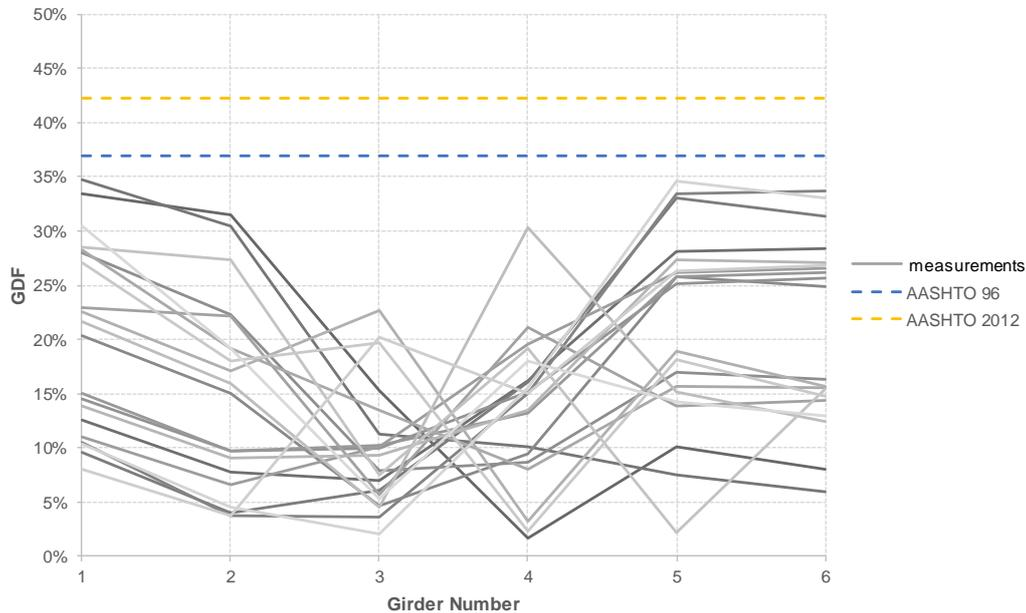
Fig. 3 GDF for single lane loading from B-WIM measurements (Pawiro Baru A Bridge, Site ID001)
