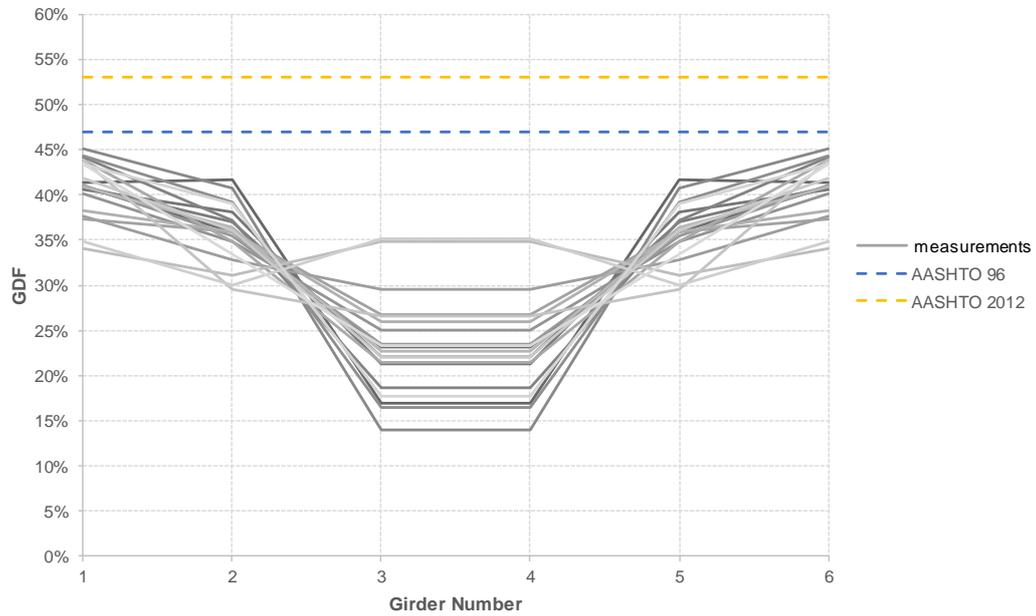
Fig. 4 GDF for two-lane loading (superposition) from B-WIM measurements (Pawiro Baru A Bridge, Site ID001)
