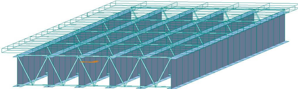
Fig. 9 3D view of the steel composite girder bridge designed with proposed GDF formula
