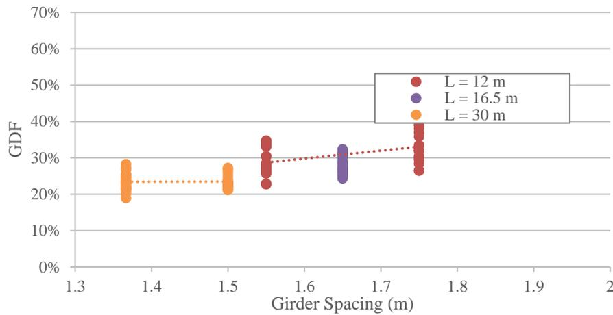
Fig. 6 Relationships between GDF and girders spacing for different span length, single lane loading
