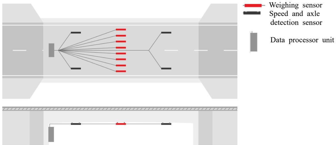
Fig. 1 Typical B-WIM system installation (CESTEL and ZAG Institute 2014)
