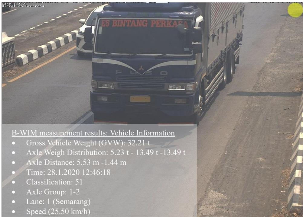
Fig. 5 Vehicle information from B-WIM measurements (Pawiro Baru A Bridge, Site ID001)
