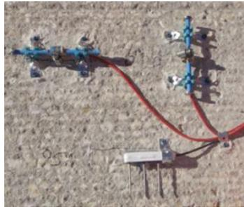
Fig. 5 Installation of Geokon4200 and GS3 on deck
