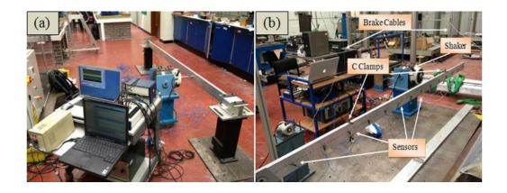
Fig. 7 Test setup for (a) Beam 3-E and (b) Beam 4-E (Asnaashari and Sinha 2014a)
